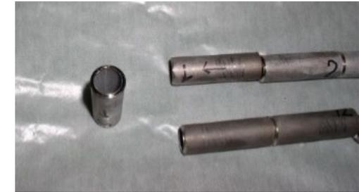
Parts of the mass transfer tube after cutting
