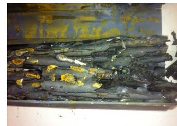
The bottom half of the assembly was an area of global cladding degradation with multiple fractures, with obvious signs of cladding material melting, the presence of longitudinal and transverse cracks on the cladding fragments left.
