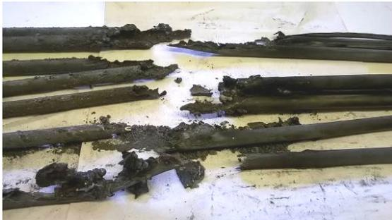
Fragments of claddings with drop-like impregnation of steel and iron were present in the area of global degradation.
