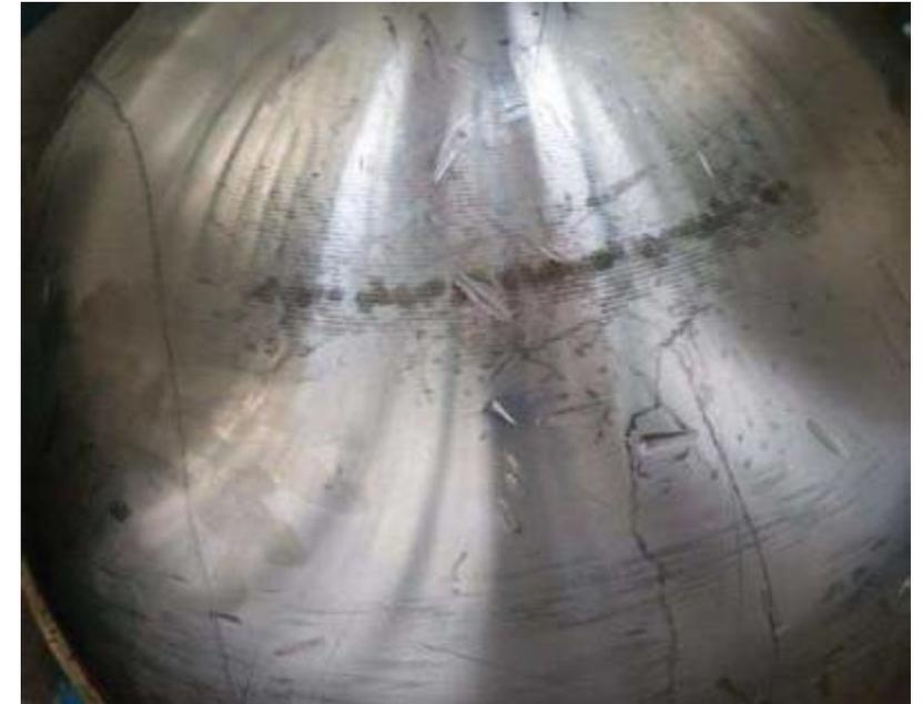
Check valve (sphere) after endurance tests
