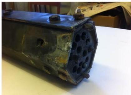
When the reaction chamber was opened, and the 19-rod assembly was removed and dismantled, it was found that sodium was present on the walls of the reaction chamber in the form of a deposit mixed with the products of its thermal interaction with the corium simulator. The assembly wrapper tube was burnt through in some places, on one of the edges the lower header was partially melted.
