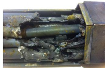
The initial configuration of the rod bundle remained the same in the outer layer, in its upper part. The inner layer of the simulators retained the initial configuration in the middle part.
