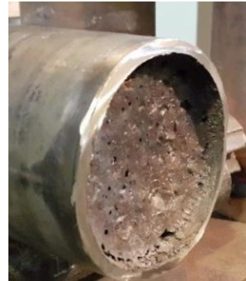
Corium simulator melt stratification into metallic (a) and ceramic (b) phases
