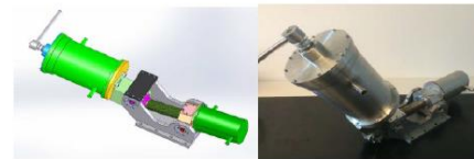
Specific tight robot mockup with 2 degrees of freedom
