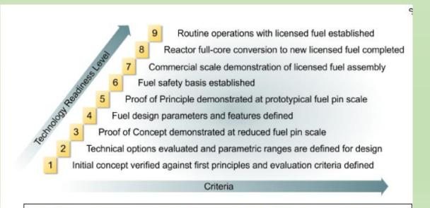
TRL 9 for Phenix type pins (Phenix, SNR300, Joyo) & same geometry with central hole (EBR2, PFR, BN800), SPX type TRL 6-7 for others concepts
