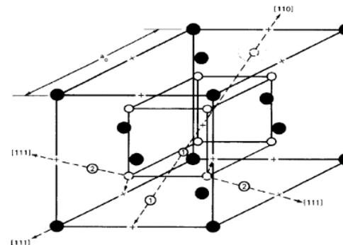
Fig. 11.5 Defect complex in  $UO_2$ . ●, uranium ions. ○, normal oxygen. ①, type 1 interstitial oxygen. ②, type 2 interstitial oxygen. ⊖, vacancy in normal oxygen site. +, interstice at center of cube formed by eight normal oxygen sites.
