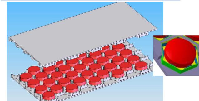
Two ceramic plates close a honeycomb structure containing cylindrical fuel pellets
