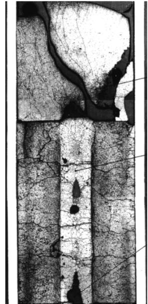
Fuel partly melt during (CABRI – E5 test)
