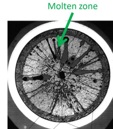
$R_{\text{melted}}/R_0 = \sim 85\%$
