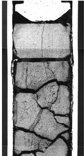
Relocation displacement induced by pellet fragmentation
