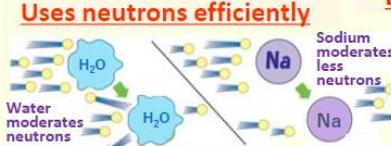
Neutrons produced in fission can be efficiently used because sodium moderates neutrons less than water does.
