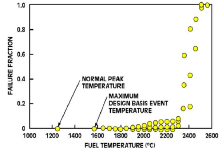
The multilayer TRISO coated particle fuel is engineered to retain fission products during normal operating conditions (~1000-1400 C) and all gas reactor licensing design basis accident events (~1600 C), including a Depressurized Cooldown Event (loss of coolant), the worse event for a HTGR.
