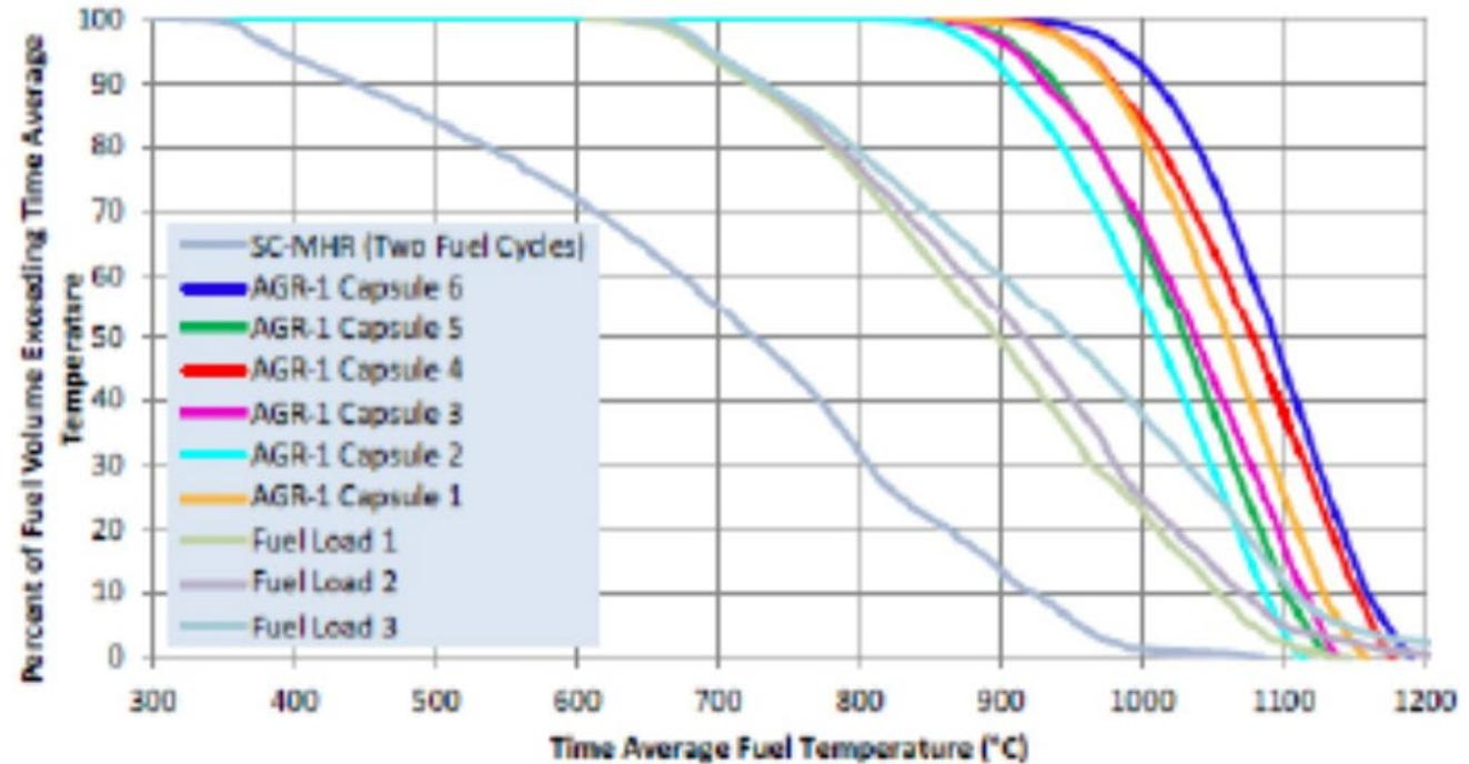
AGR Experiments Fuel Temperature “waterfall” vs. TRISO Fuel Temperatures in HTGRs
