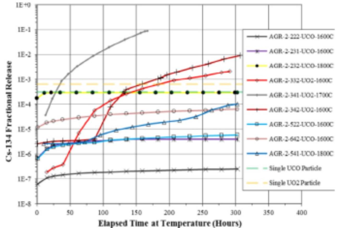
AGR-2 UCO TRISO fuel has successfully survived 300 hour safety tests at 1600 C, 1700 C, and 1800 C.
