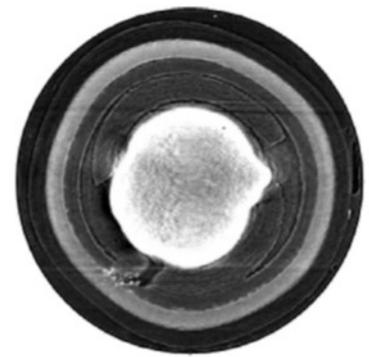
X-ray tomogram of an irradiated AGR-1 particle with fission product attack on its SiC layer
