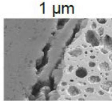
SEM Image of Buffer Kernel Interface in Particles
