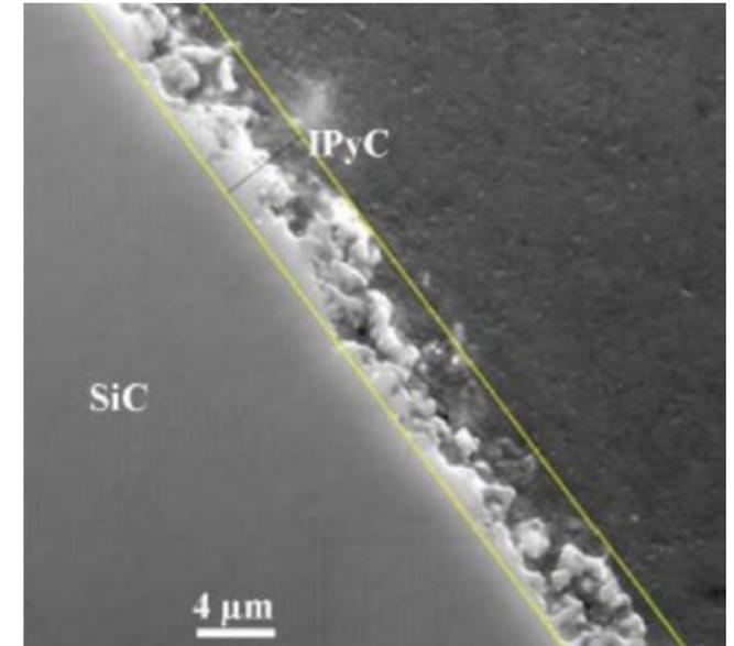
SEM image SiC-IPyC interlayer thickness marked between the yellow lines
