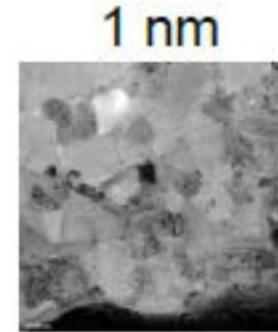
High resolution FIB/TEM images of precipitate near IPyC/SiC Interface
