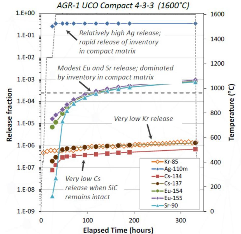
AGR TRISO fuel has successfully survived 300+ hour safety tests at 1600 C, 1700 C, and 1800 C.
