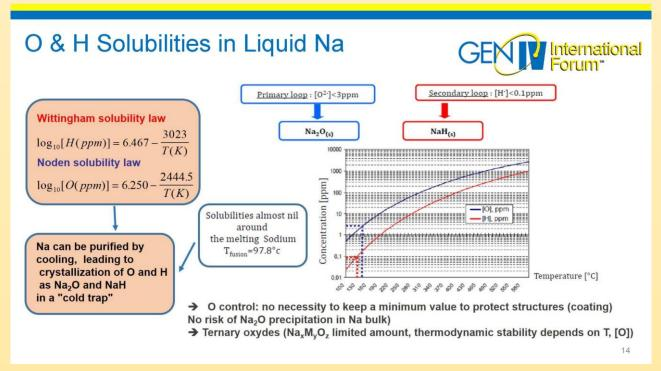
The principle of purification in a cold trap is explained. Sodium can be purified by cooling, leading to crystallization of O and H as Na<sub>2</sub>O and NaH in a "cold trap". The cooled sodium is then heated up again for operation.
