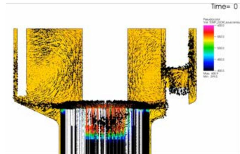
*Modelling of an accidental scenario with loss of the primary pump of ASTRID reactor, without control rod protection (ULOF). Natural convection is leading to a stabilised sodium flow in the core allowing core assemblies cooling and avoiding a severe accident situation (no core or fuel melting). CEA/Saclay studies*
