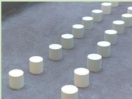
ThorEnergy@ IFE, Norway, (Th, Ce) 2 O 7 Irradiation tests at OECD Halden Reactor
