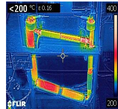
IR image during heater testing - inside of the loop is at 700°C
