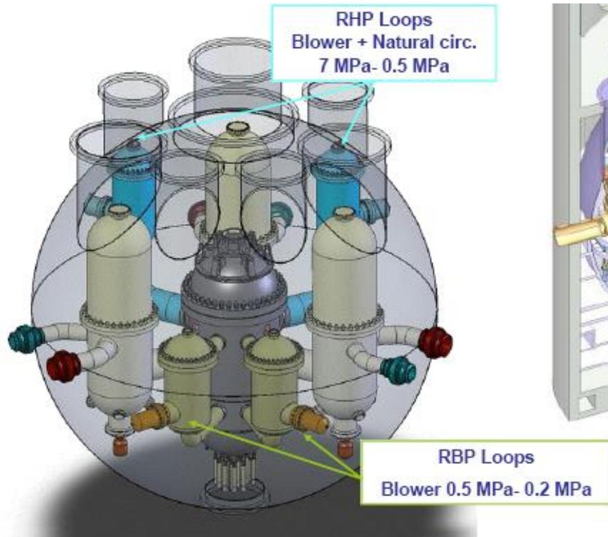
Figure 2: GFR Primary and DHR system inside the guard containment
