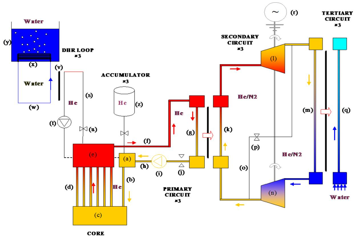
Figure 9: GFR system nodalisation diagram
