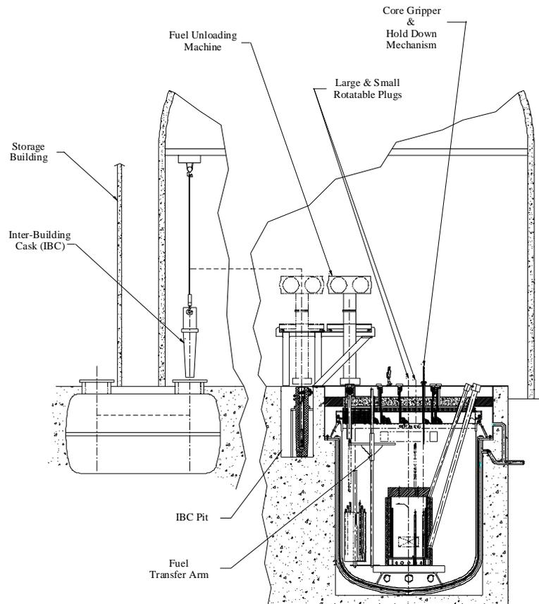
**Figure A.9. Transfer of fuel assemblies in and out of the primary tank/reactor building**
