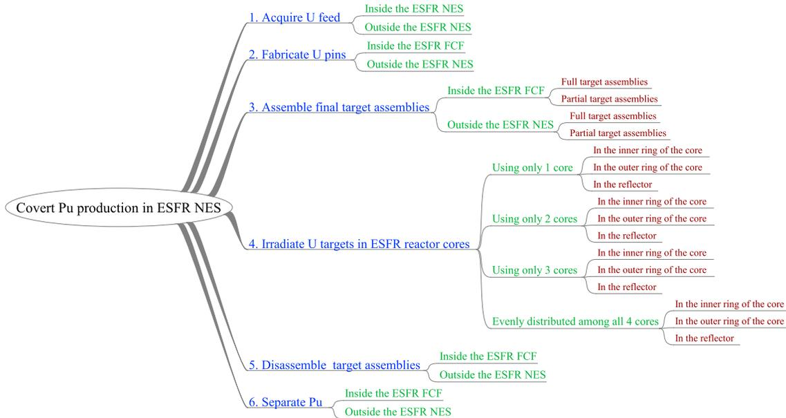
**Figure D.2-2: Covert Pu production in ESFR NES: Pathway identification.**
