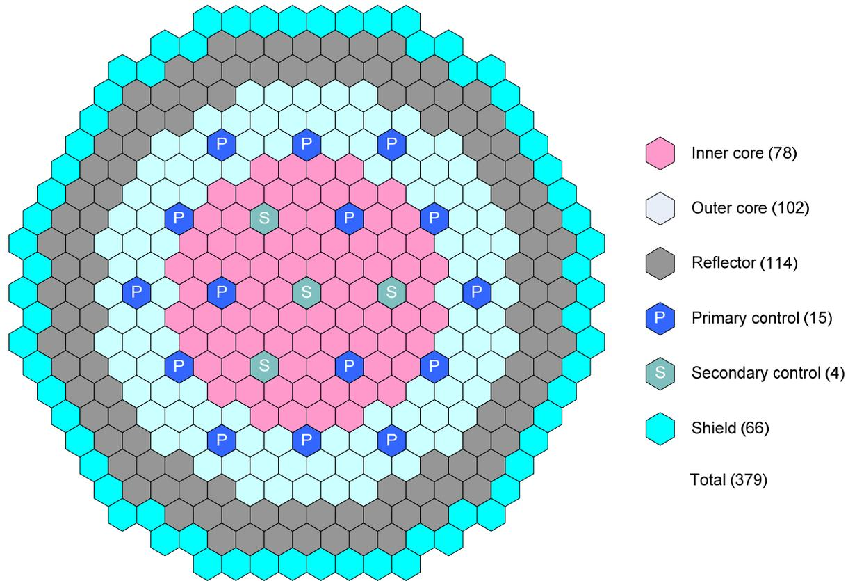
**Figure A.19. 1000 MW<sub>th</sub> Reactor Radial Core Layout**
