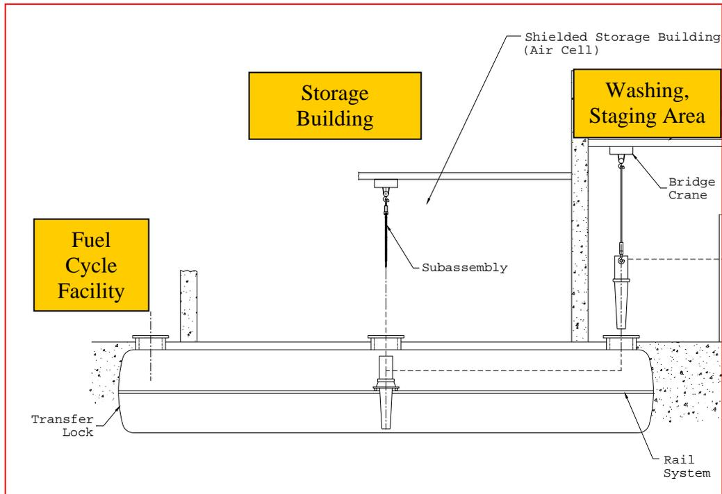
**Figure A.10. Transfer of fuel assemblies from washing area to the storage building and the fuel processing facility.**
