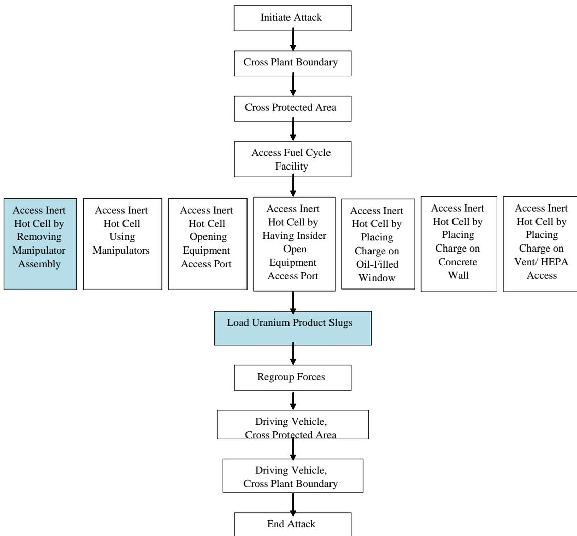
**Figure 6.4:** Adversary Sequence Diagram for Theft of TRU/Uranium Product (in process cell)
