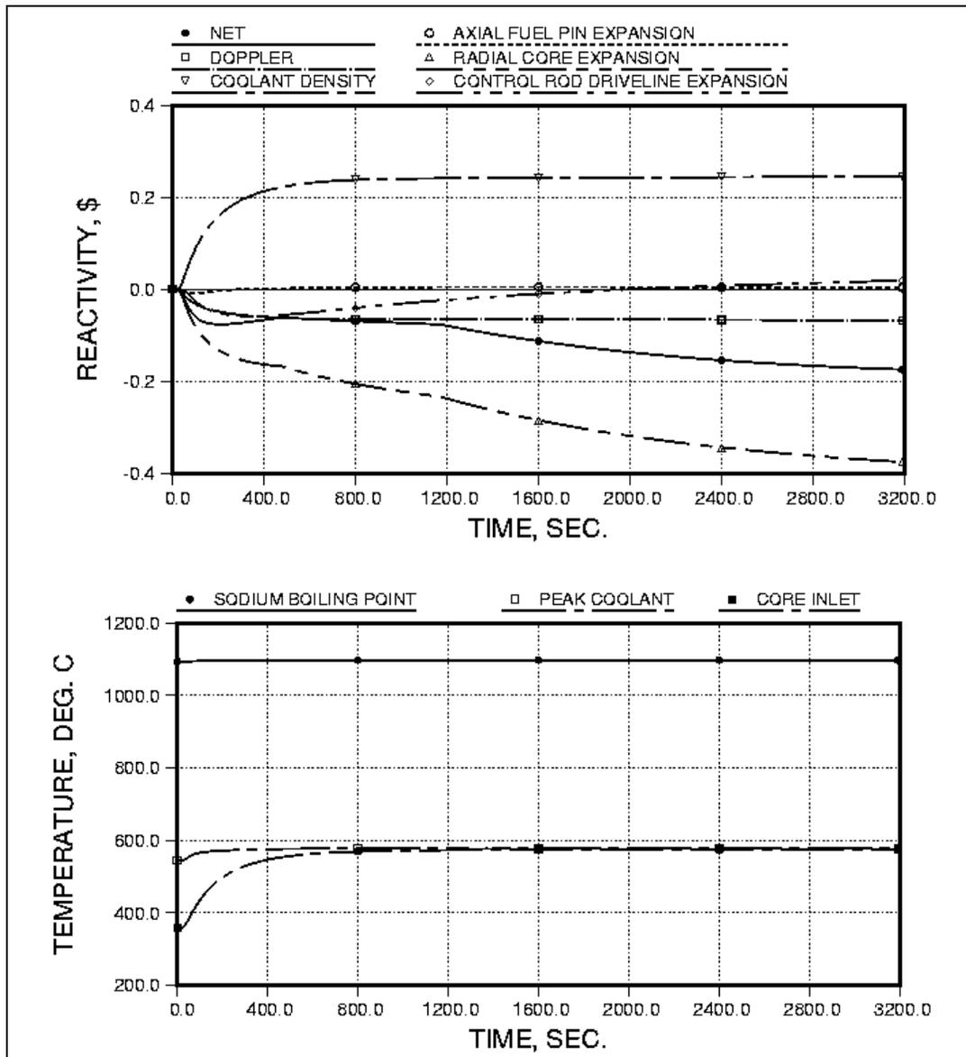
**Figure A.18. Reactivity and Temperature History for a ULOHS Transient – 3500 MWe Plant, Reference [A.3].**
