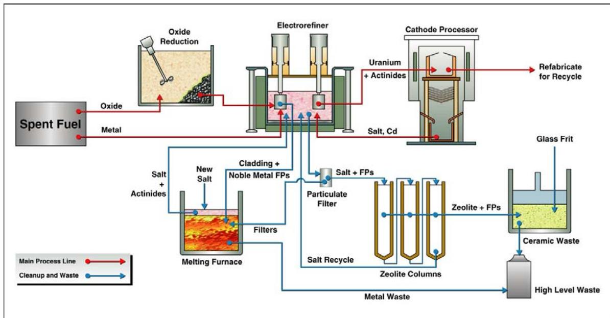
Figure A.12. Diagram of the fuel cycle facility operations.
