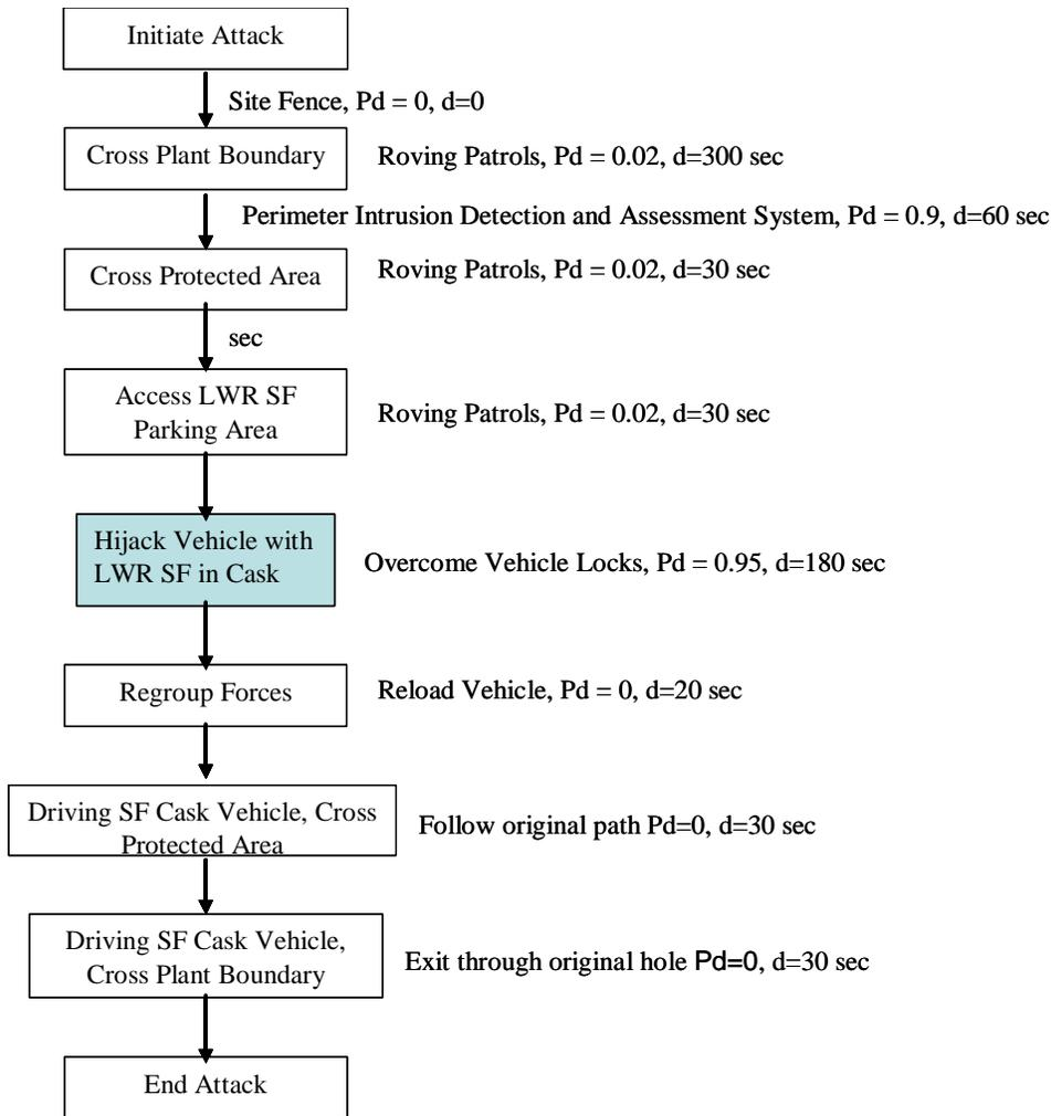
**Figure D.4-19. Annotated Adversary Sequence Diagram for Theft of SF Shipping Casks**
