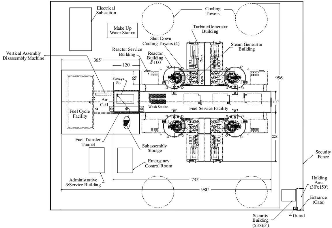
**Figure D.4-2. ESFR Nuclear Energy System Site Layout**
