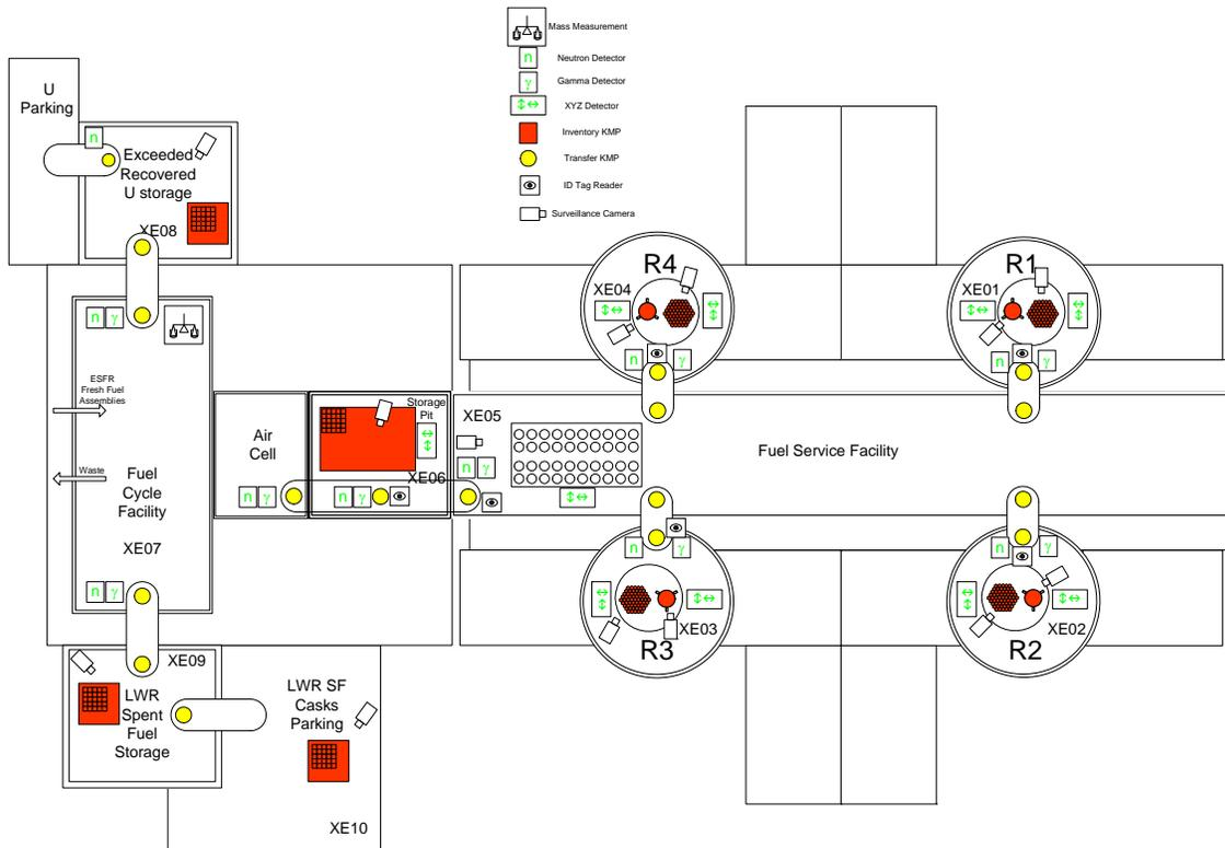
Figure B.3. ESFR Nuclear Energy System MBAs and SPs. Note that: a) Waste and fresh fuel assemblies input to the FCF are not further considered.
