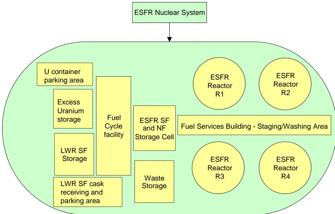
Figure A.1. Diagram of ESFR Nuclear System Elements.
