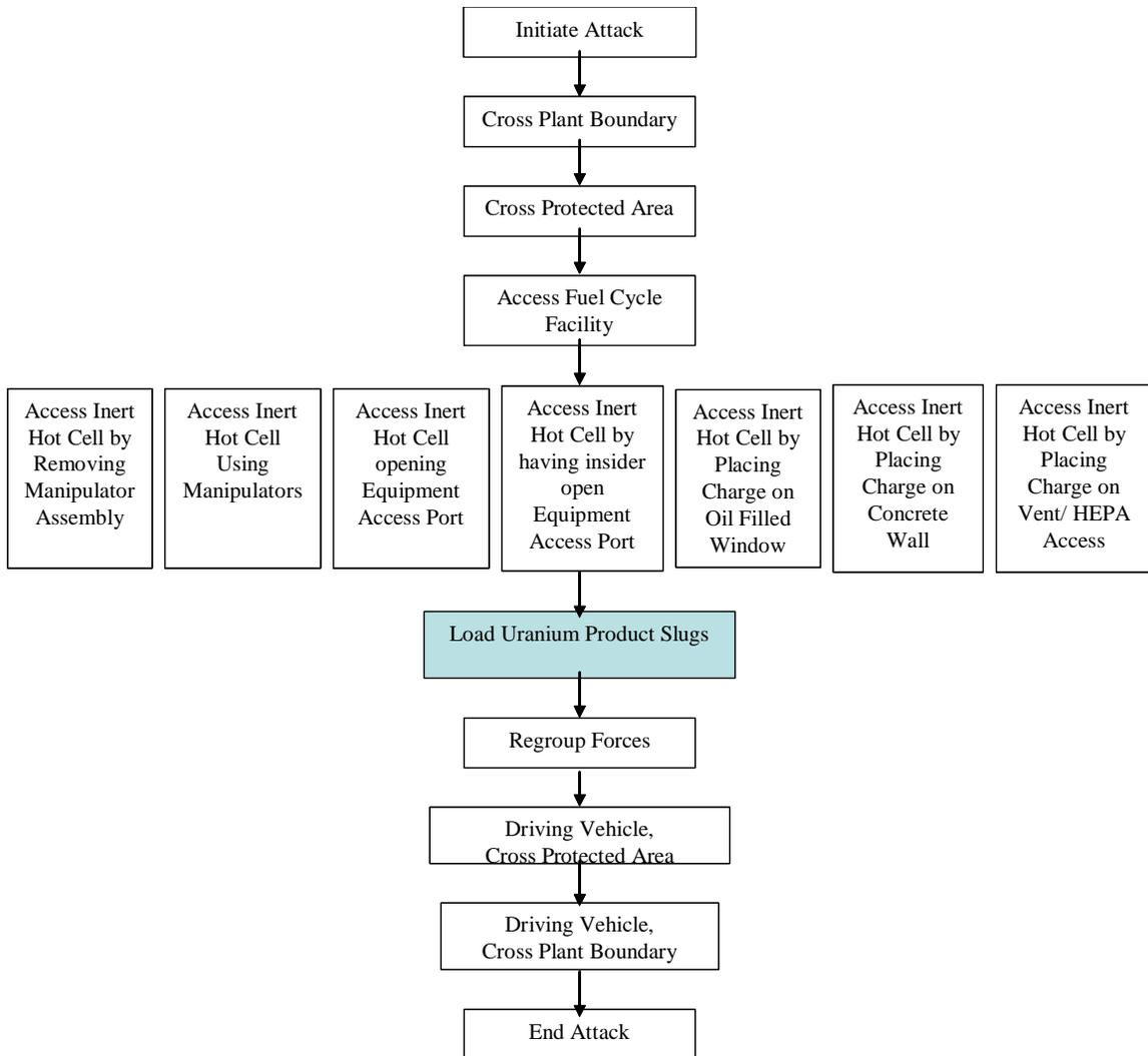
**Figure D.4-9. Adversary Sequence Diagram for Theft of Uranium Product (in Process Cell)**
