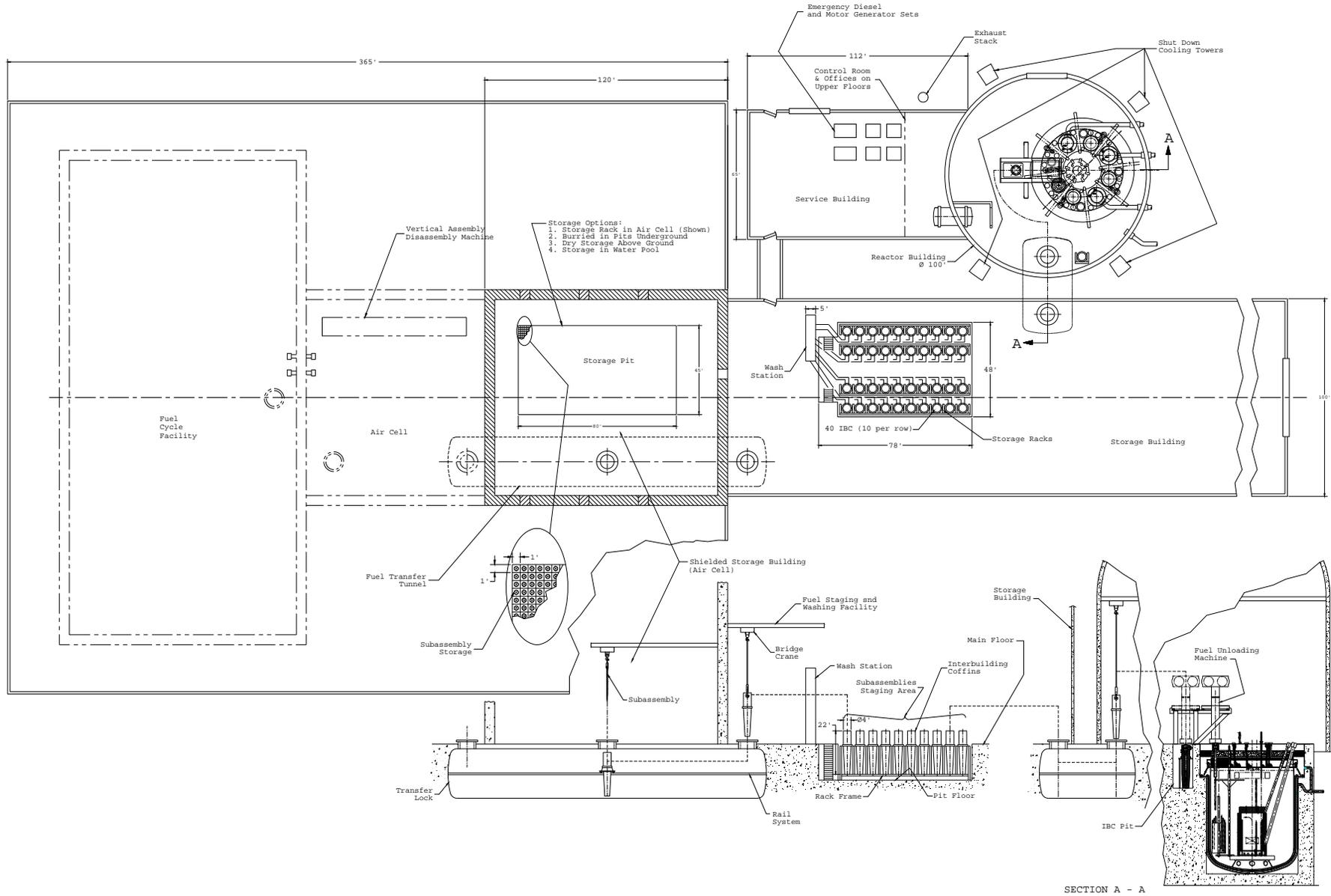
Figure A.7. Fuel Handling System - Plant Layout
