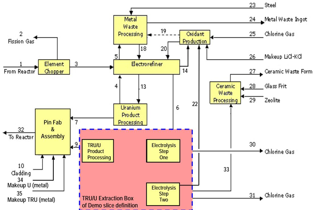
**Figure A.14. Process Overview for Two-Stage Electrolysis Option**
