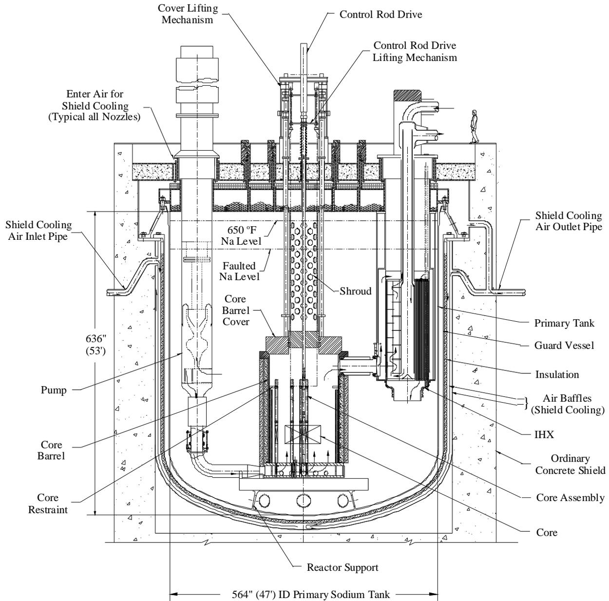
**Figure A.4. Elevation View of the Reactor Primary Systems.**
