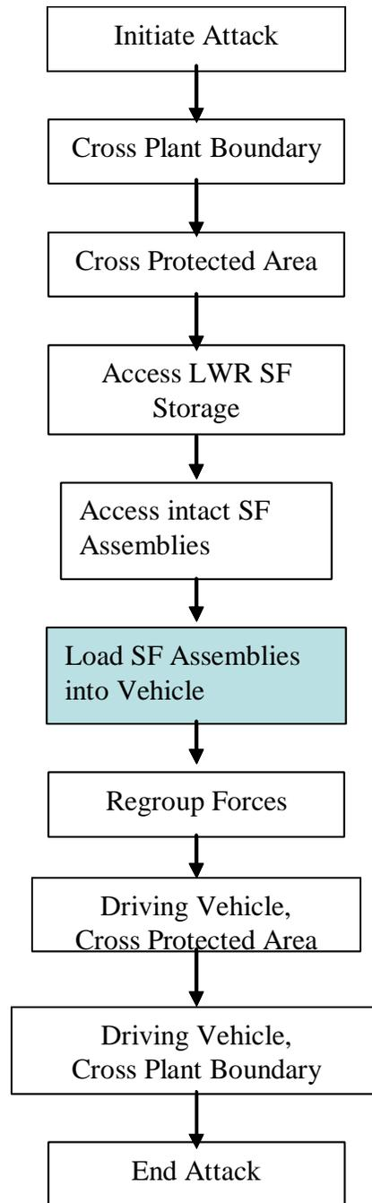
**Figure D.4-5. Adversary Sequence Diagram for Theft of LWR Spent Fuel in LWR SF Storage Area**
