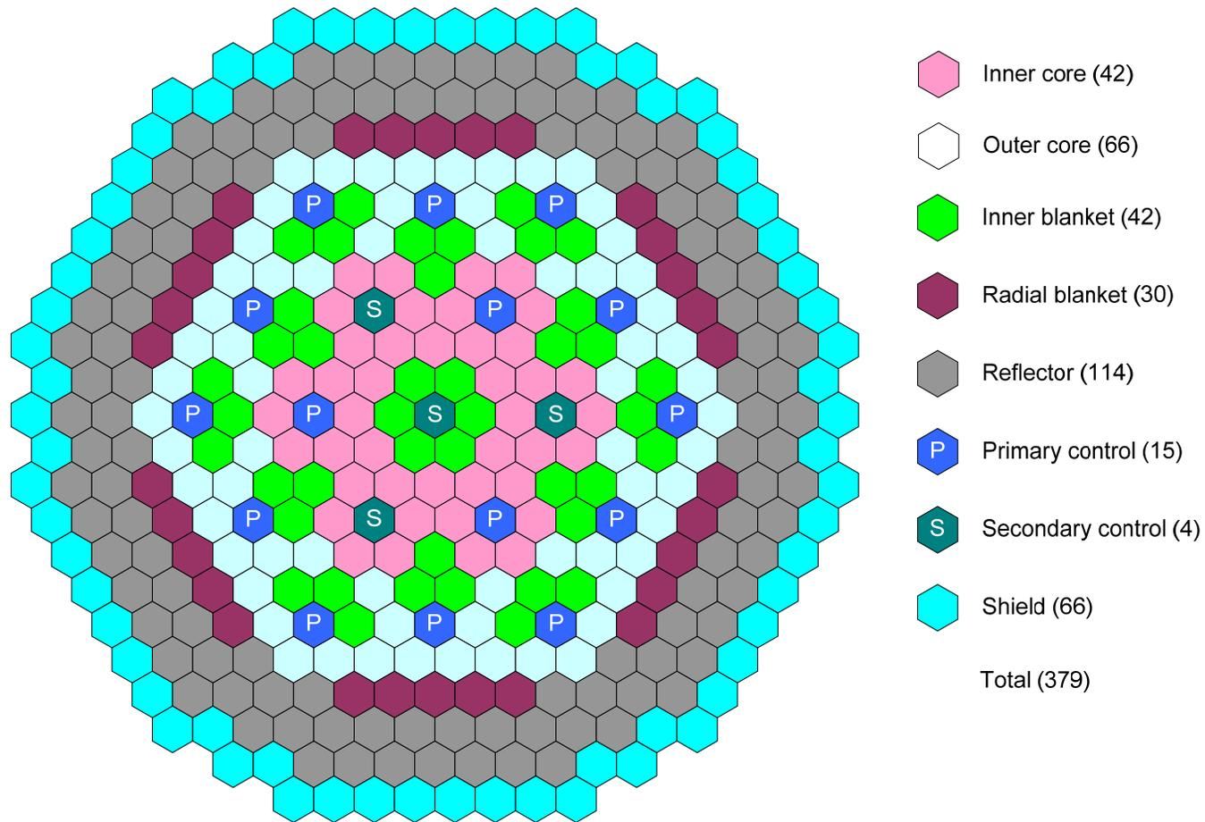
Figure A.20. 1000 MW<sub>th</sub> Reactor Radial Core Layout Design Variation 3: TRU CR=1.12
