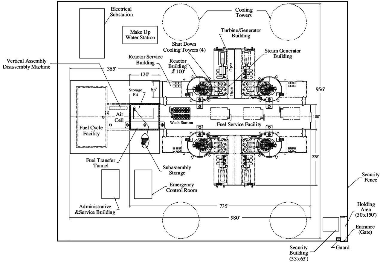
Figure 2.3: Possible Overall Site Plan
