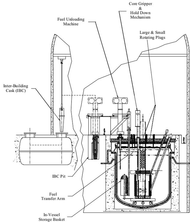
Figure B.4. Detail of the Reactor Core and related fuel transfer system [B.1].
