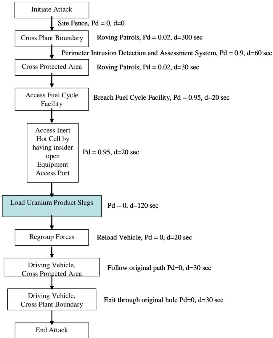
**Figure D.4-20. Annotated Adversary Sequence Diagram for Theft of Uranium Product Slugs**
