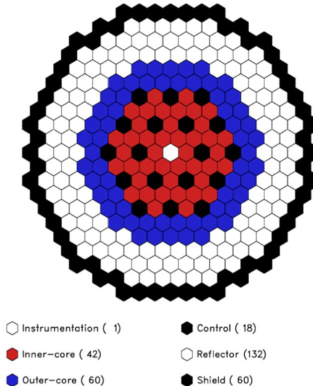
**Figure A.5. Baseline 800 MW<sub>th</sub> Reactor
