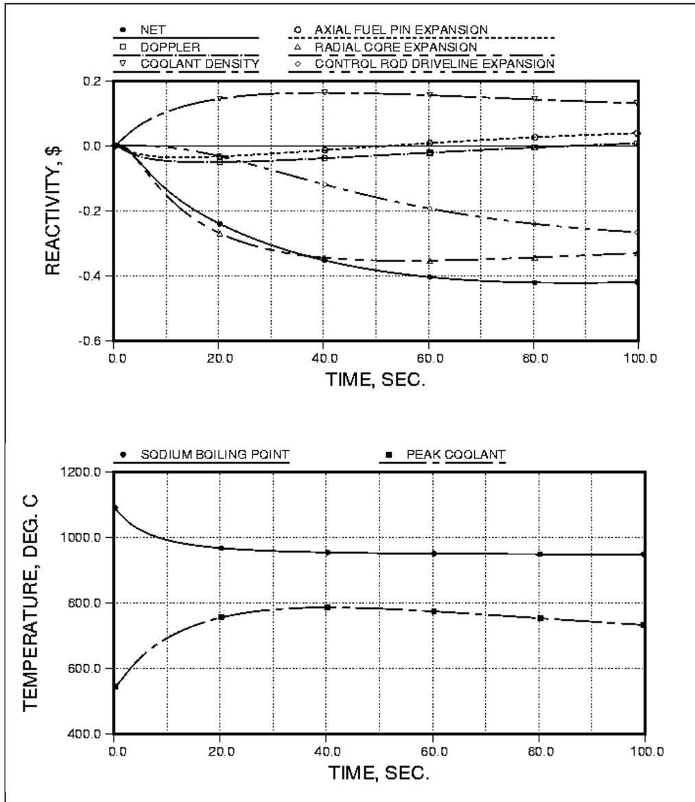
Figure A.17. Reactivity and Temperature History for a ULOF Transient – 3500 MWe Plant, Reference [A.3].
