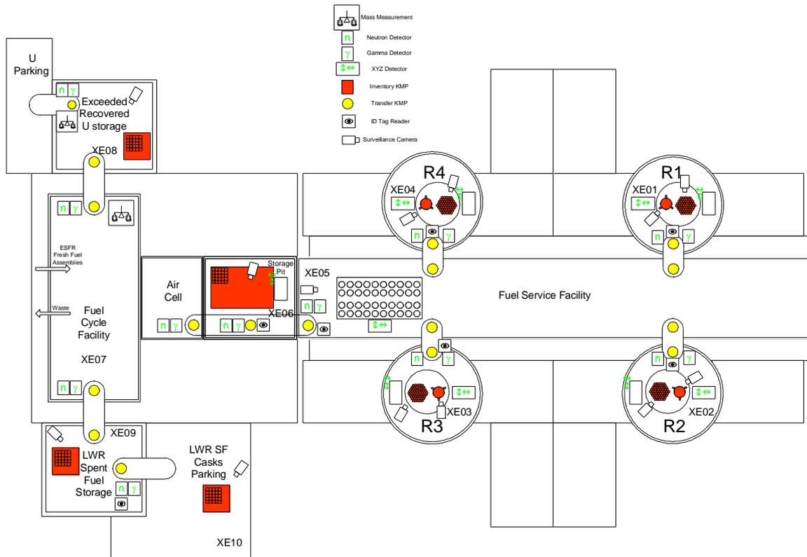
Figure 7: Safeguards system developed for the Example Sodium Fast Reactor (ESFR), object of the GIF PRPP Case Study [30]. The site co-locates 4 nuclear power units, a recycling facility and related fresh and spent fuel storage.
