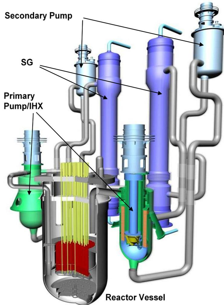
Figure 1: Conceptual Plant Layout of the JAEA Sodium Fast Reactor (JSFR) [12].
