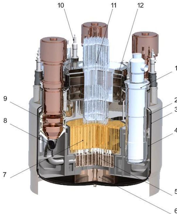
1 – Intermediate Heat eXchanger; 2, 3 – main and guard vessels respectively; 4 – supporting structure; 5 – inlet plenum; 6 – core catcher; 7 – core; 8 – pressure pipeline; 9 – Main Coolant Pump-1; 10 – Decay Heat eXchanger; 11 – Control Rod Driveline Mechanism; 12 – rotating plugs
