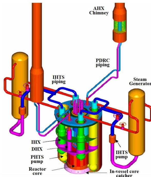
Figure 2: KALIMER-600 System Configuration [19].
