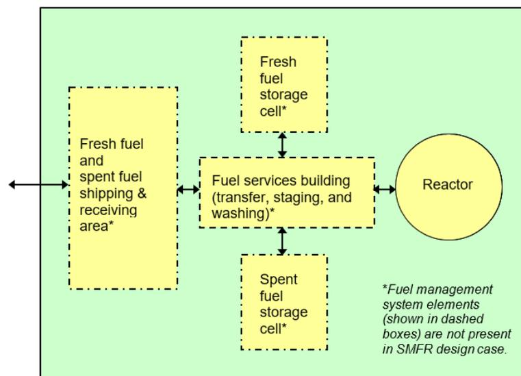
Figure 6: SFR System Elements containing nuclear material.
