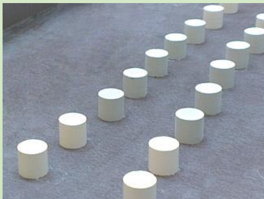
ThorEnergy@ IFE, Norway, (Th, Ce)O 2 Irradiation tests at OECD Halden Reactor
