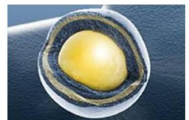
TRISO coated particle fuel
