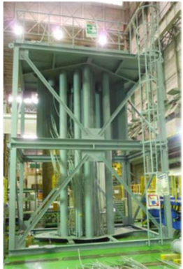
Mockup of above core structure
