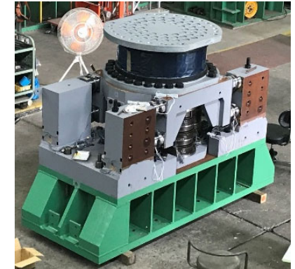
1/2 scaled mockup of 3D seismic isolation system
